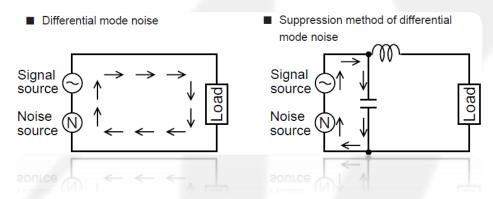
Seen above is that the inductance in your signal cable, plus added mutual capacitance, effectively created a second order low pass filter. It's the amount of inductance and capacitance that decides how and what higher frequencies will be filtered out. Wires have some self-induction and two wires put in a cable (not a vacuum) will always have some mutual capacitance. Be careful what you choose to add to your system...
